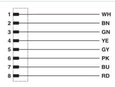
Contact assignment of the M12 plug
