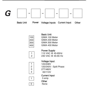
For other Voltage and Current Inputs, contact Simpson Electric Company
