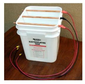
Hang 4 anodes on each anode bus bar, making sure they are evenly spaced across the bars.
