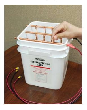
Attach the bus bar wires to the rectifier, the red wires from the anode bus bars to the positive (+) terminal, and the black wire from the cathode bus bar to the negative (-) terminal.
