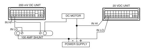
LO terminal. The Mini-Max units will indicate the power supply voltage and load current of the motor.
