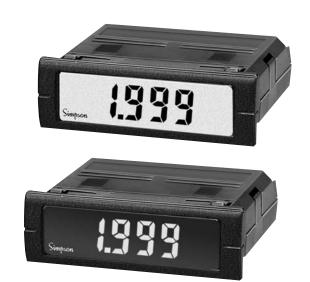
Simpson's Mini-Max Current Indicators provide high quality, accuracy and reliability in a compact, 60mm deep case. Units offer 3-1/2 digit, 0.5" (12.7mm) LCD display and are available with a bright red, negative image backlight option. All units feature user-selectable decimal point, auto zero and limited scaling capabilities.
