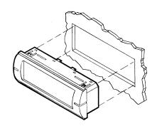
No mounting hardware required, snaps right into panel!
