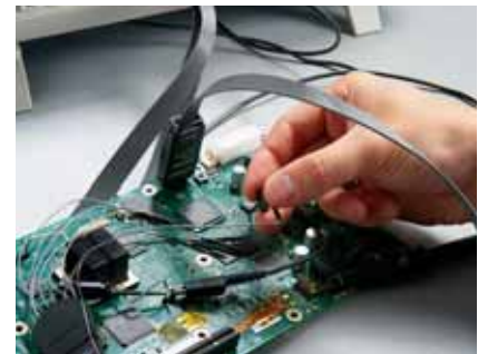
The P6316 digital probe for MSO2000 Series simplifies connection to the device-under-test
