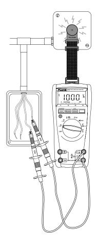
Get our ToolPak $^{^{\text{\tiny M}}}$  and free both hands to finish jobs faster and easier. You get a powerful magnet, a loop hanger and two straps—for hanging your meter from almost anything while you work.
