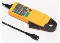
The i310s current probe is based on Hall Effect technology for use in measurement of both DC and AC current. The i310s may be used in conjunction with oscilloscopes and other suitable recording instruments for accurate nonintrusive current measurement.
