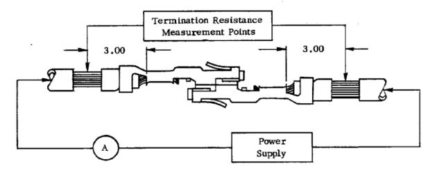
Notes: 1. A I foot minimum length of continuous lead for heat dissipation.
