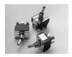
The H-Series toggle switches are heavyduty, high voltage, high amperage, threepole switches. These switches have a slow-make. slow-break contact mechanism, are AC rated to 600V, and are available in a wide range of ratings, circuits, terminations and bushing/toggle configurations.
