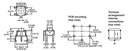
Note: Terminal numbers are not indicated on this switch. With the switch turned over so that the logo mark "OMRON" is visible on the upper part of the rear side of the switch base, the terminal on the right of the logo mark is numbered "1" and that on the bottom right is "3." Accordingly, two terminals on the left side are numbered "2" and "4" respectively.
