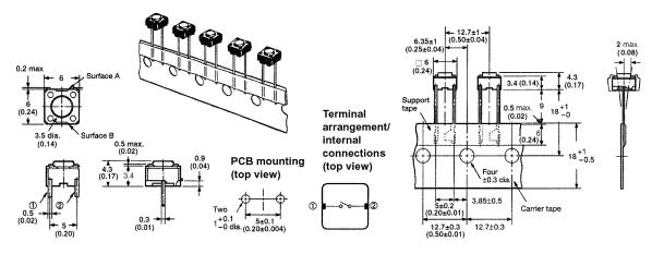
Note: The tape is random between surface A and surface B.
