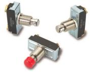
The 170/172-Series pushbutton switches are single pole, high amperage switches suitable for shallow back panel applications. These switches are momentary action and require an actuation force of 2.5 lbs. The 170/172-Series switches are equipped with a slow-make, slow-break contact mechanism and are rated at 15 amps at 125VAC.
