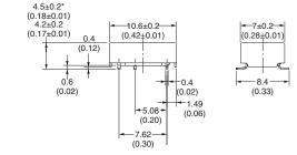
Note: Each value has a tolerance of ±0.3 mm. \*This dimension effective April, 2005.
