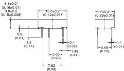
Note: Each value has a tolerance of ±0.3 mm. \*This dimension effective April, 2005.
