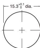
Panel Cutout Dimension Panel thickness = 1 to 4 mm
