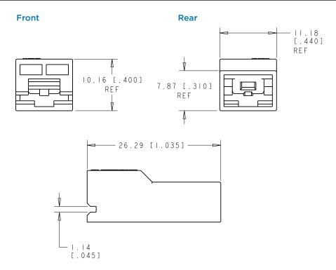
**Tyco Electronics** I .312 Series FASTON Receptacle Connectors
