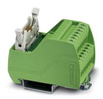
VARIOFACE module, with screw connection and flat-ribbon cable plug connector, for mounting on NS 32 or NS 35/7.5, with pin strip and short and long locking latches for socket strips, 16-pos.
