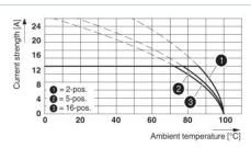
Derating diagram for conductor cross-section  $2.5 \text{ mm}^2$ ; reduction factor = 0.8
