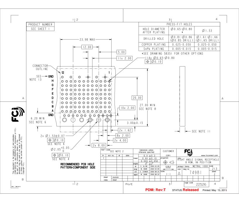
10. SEE GS-20-018 FOR APPLICATION OF CONNECTOR TO PCB.
