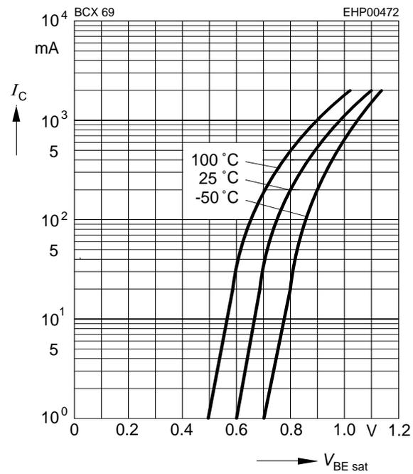
**Collector current  $I_C = f(V_{BE})$**
