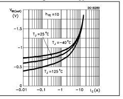
Figure 10. Base-emitter on voltage for NPN type
