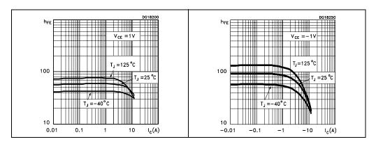
Figure 4. DC current gain for NPN type Figure 5. DC current gain for PNP type
