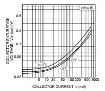
Fig.6 Collector-emitter saturation voltage vs. collector current
