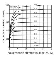
Fig.2 Ground emitter output characteristics
