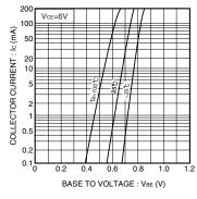
Fig.1 Ground emitter propagation characteristics
