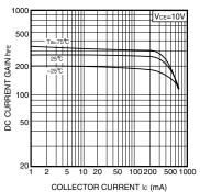
Fig.4 DC current gain vs. Collector currnet (II)
