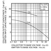
Fig.7 Input-and-output capacity vs.voltage characteristic
