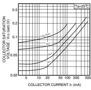
Fig.5 Collector-emitter saturation voltage vs. Collector current
