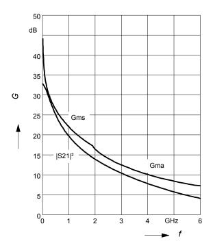
Power gain  $G_{ma}$ ,  $G_{ms} = f(V_{CE})$  $I_{C} = 20 \text{ mA}$
