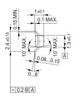
1) Lead width can be 0.6 max. in dambar area
