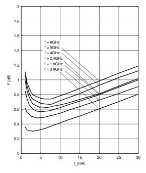
**Minimum noise figure**  $NF_{min} = f(f)$  $V_{CE} = 3V, Z_S = Z_{Sopt}$
