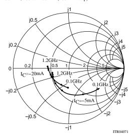
$\begin{array}{l} S12e: V_{CE} \!\!=\!\! -10V \\ f \!\!=\!\! 100 MHz, 200 \text{ to } 1200 MHz (200 MHz \text{ step}) \end{array}$
