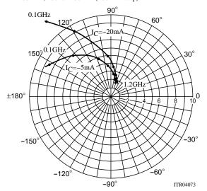
$\begin{array}{l} S22e: V_{CE}\!\!=\!\!-10V \\ f\!\!=\!\!100MHz, 200 \text{ to } 1200MHz (200MHz \text{ step}) \end{array}$
