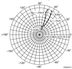
$\label{eq:solution} \begin{array}{l} \textbf{S parameter} \\ \text{S21e}: V_{CE} = -10V \\ \text{f=}100\text{MHz}, 200 \text{ to } 1200\text{MHz} (200\text{MHz step}) \end{array}$
