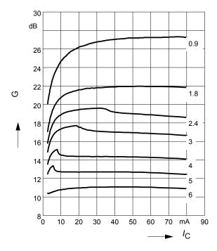
Minimum noise figure  $NF_{min} = f(I_C)$  $V_{CE} = 2 V, Z_S = Z_{Sopt}$
