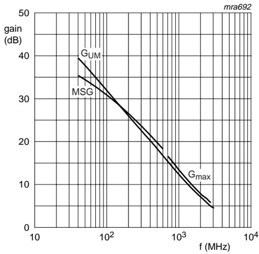
$V_{CE} = 8\text{ V}; I_C = 10\text{ mA}.$
