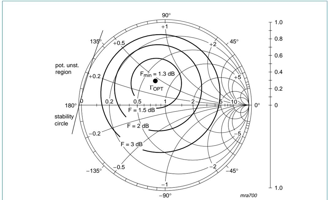
$Z_o = 50 \Omega$ ;  $V_{CE} = 8 \text{ V}$ ;  $I_C = 10 \text{ mA}$ ;  $f = 900 \text{ MHz}$ .
