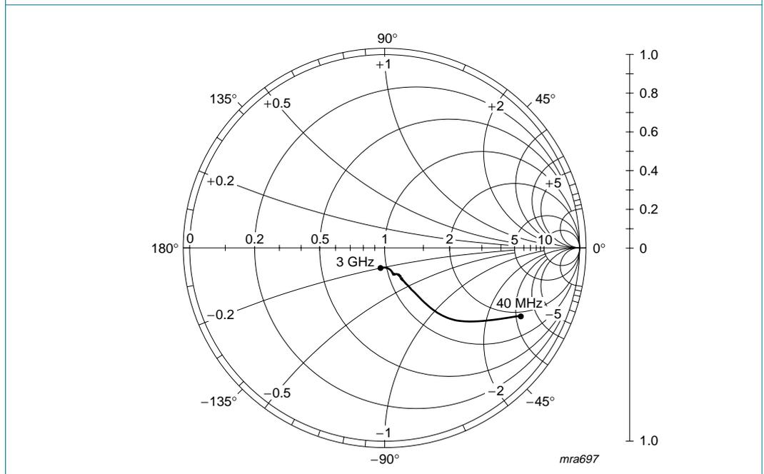
$V_{CE} = 8\text{ V}; I_C = 40\text{ mA}; Z_o = 50\ \Omega$ .
