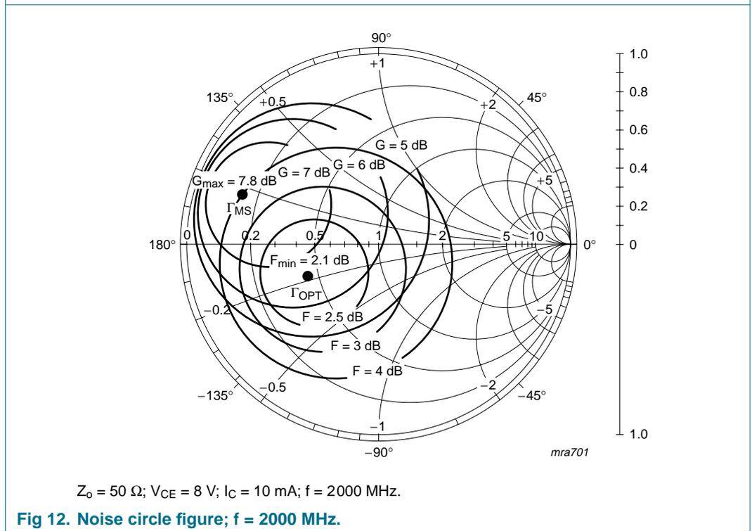
$Z_o = 50 \Omega$ ;  $V_{CE} = 8 \text{ V}$ ;  $I_C = 10 \text{ mA}$ ;  $f = 2000 \text{ MHz}$ .
