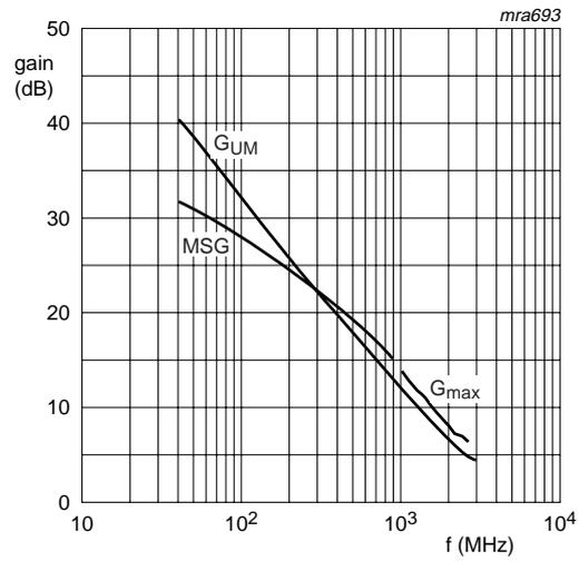
$V_{CE} = 8\text{ V}; I_C = 40\text{ mA}.$
