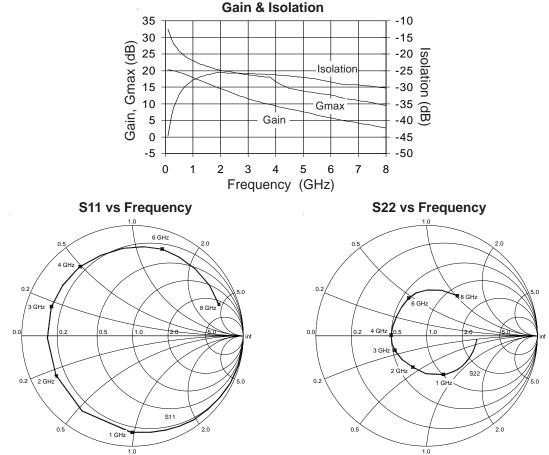
De-embedded S-Parameters ( $Z_s = Z_L = 50$  Ohms,  $V_{DS} = 8V$ ,  $I_{DS} = 100$ mA, 25°C)
