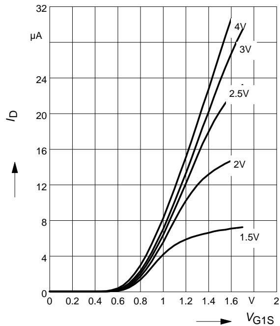
**Drain current  $I_D = f(V_{GG})$  amp.A=amp.B**
