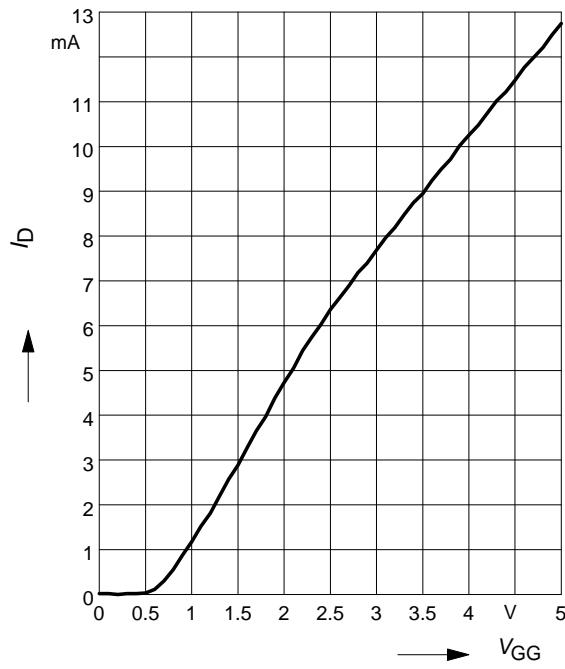
**Drain current  $I_D = f(V_{GG})$**
