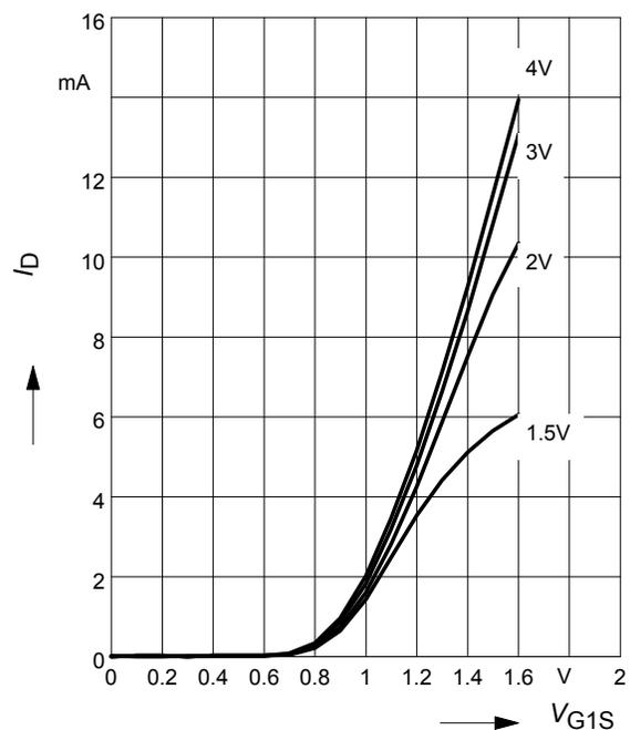
**Drain current  $I_D = f(V_{GG})$  amp. A**
