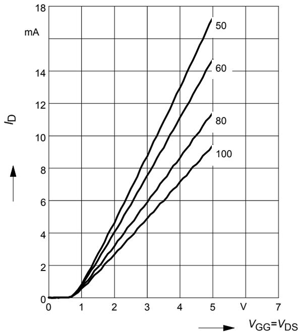
**Drain current  $I_D = f(V_{GG})$**
