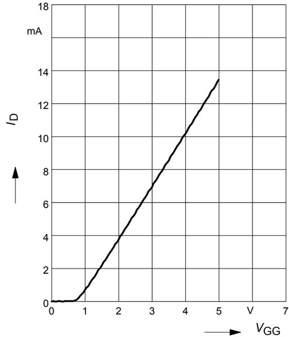
**Drain current  $I_D = f(V_{GG})$**
