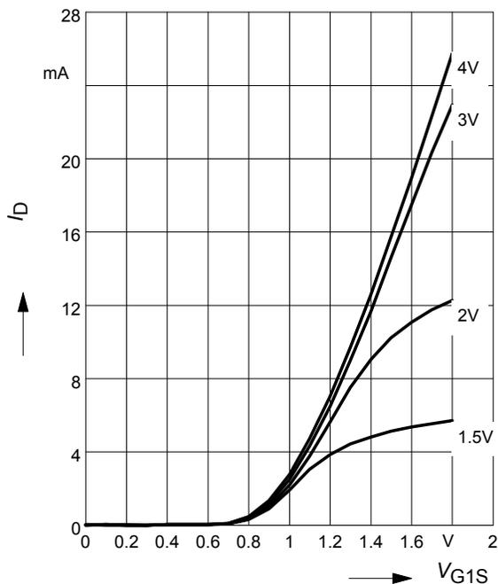
**Drain current  $I_D = f(V_{G1S})$**
