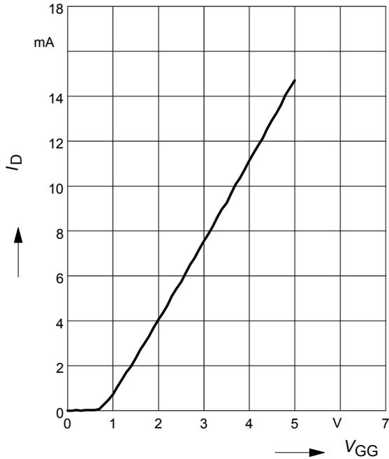
**Drain current  $I_D = f(V_{GG})$  amp. B**
