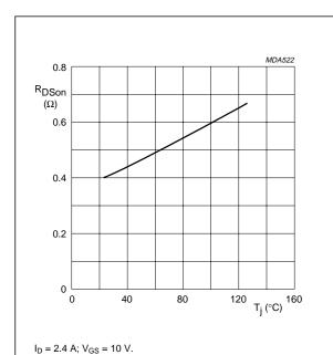
Fig.6 Drain-source on-state resistance as a function of junction temperature; typical values per section.
