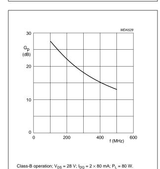
Fig.15 Power gain as a function of frequency; typical values per section.
