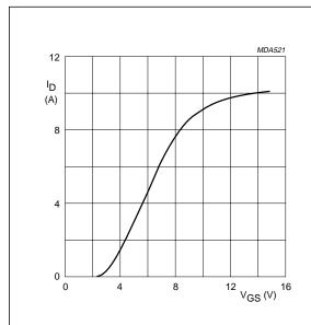
$V_{DS} = 10 \text{ V}; T_j = 25 \text{ }^{\circ}\text{C}.$
