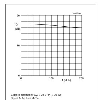
Fig.15 Power gain as a function of frequency, typical values.
