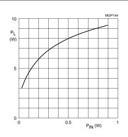
Class-B operation;  $V_{DS}$  = 28 V;  $I_{DQ}$  = 10 mA;  $R_{GS}$  = 47  $\Omega$ ; f = 175 MHz.
