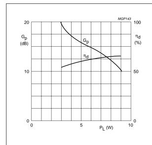
Class-B operation;  $V_{DS}$  = 28 V;  $I_{DQ}$  = 10 mA;  $R_{GS}$  = 47  $\Omega$ ; f = 175 MHz.
