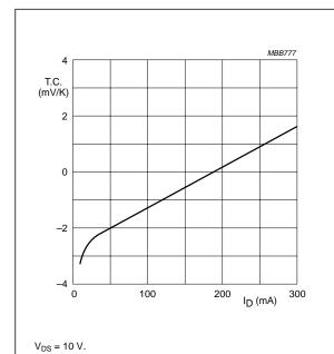
Fig.4 Temperature coefficient of gate-source voltage as a function of drain current, typical
