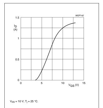
Fig.5 Drain current as a function of gate-source voltage, typical values.
