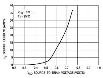
Figure 10. Diode Forward Voltage versus Current
