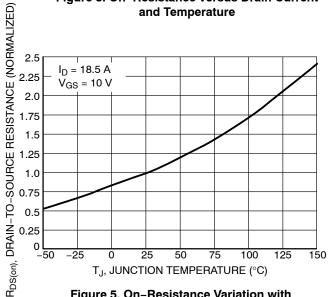
Figure 5. On-Resistance Variation with **Temperature**
