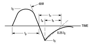
Figure 14. Diode Reverse Recovery Waveform
