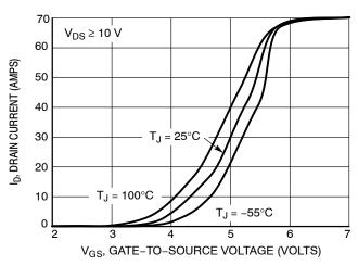
Figure 2. Transfer Characteristics
