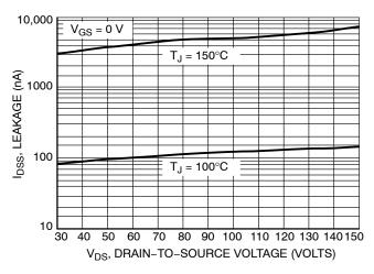
Figure 6. Drain-to-Source Leakage Current versus Voltage
