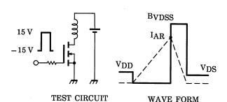
$R_{G} = 25 \Omega$  $V_{DD} = 25 V, L = 339 \mu H$  IT WAVE FORM  $EAS = \frac{1}{2} \cdot L \cdot I^{2} \cdot \left( \frac{BVDSS}{BVDSS - VDD} \right)$
