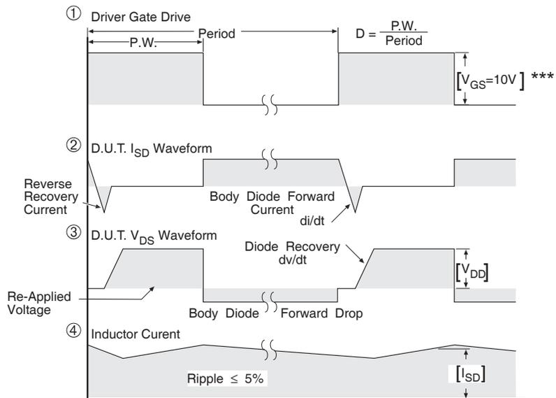
\*\*\*  $V_{GS} = 5.0V$  for Logic Level and 3V Drive Devices
