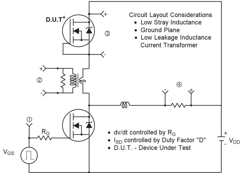
\* Reverse Polarity of D.U.T for P-Channel
