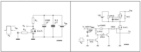
Figure 15. Test circuit for inductive load switching and diode recovery times
