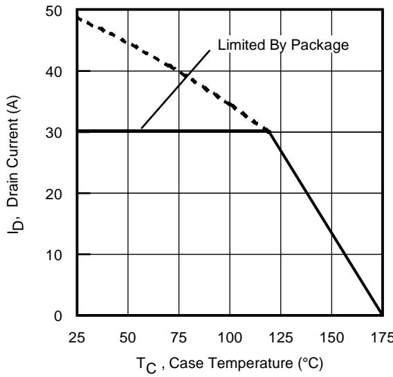
**Fig 9.** Maximum Drain Current vs.
