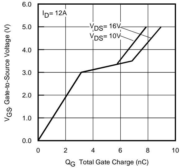
**Fig 6.** Typical Gate Charge vs.
