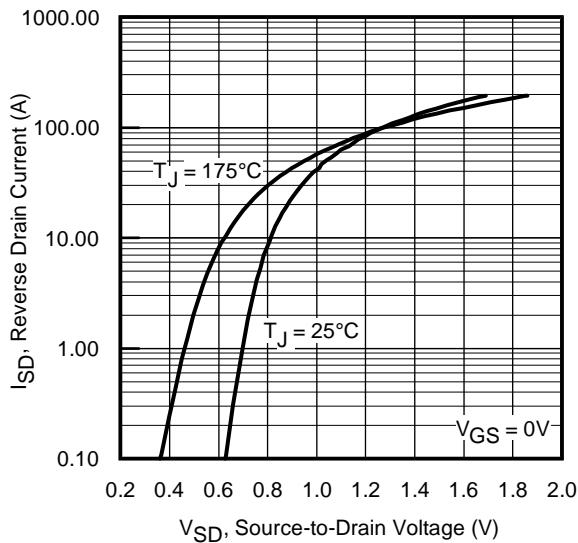
**Fig 7.** Typical Source-Drain Diode
