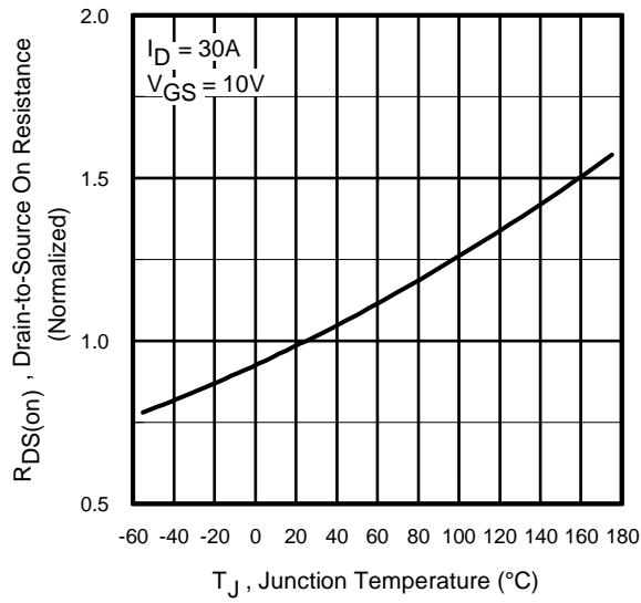
**Fig 4.** Normalized On-Resistance
