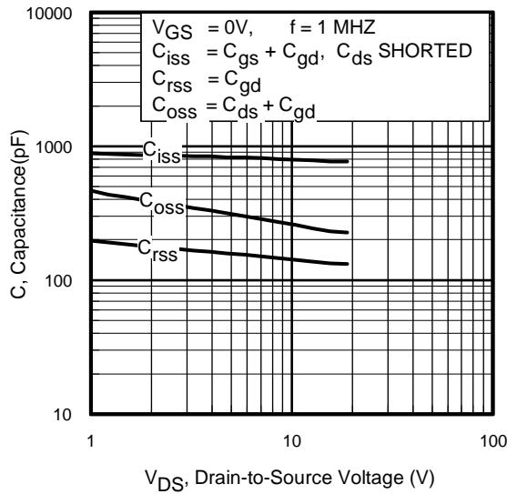
**Fig 5.** Typical Capacitance vs.
