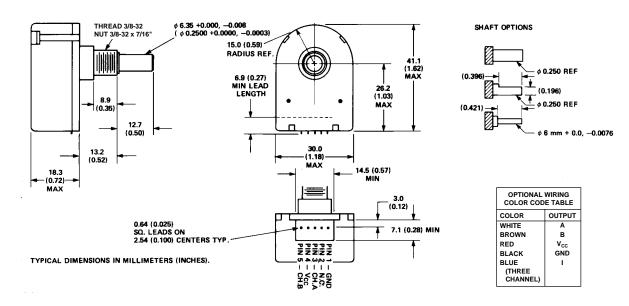
\*Note: For the HEDS-5700, Pin #2 is a No Connect. For the HEDS-5740, Pin #2 is Channel I, the index output.
