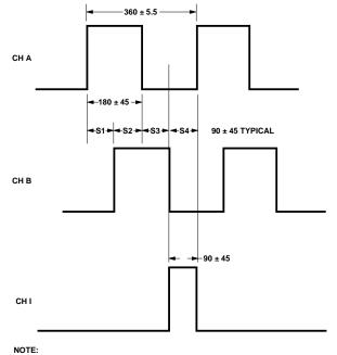
NOTE: ALL VALUES ARE IN ELECTRICAL DEGREES, WHERE  $360^\circ e = 1$  CYCLE OF RESOLUTION. ERRORS ARE WORST CASE OVER ONE REVOLUTION. CH B LEADS CH A FOR COUNTERCLOCKWISE ROTATION. CH A LEADS CH B FOR CLOCKWISE ROTATION.
