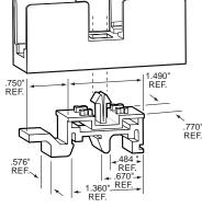
Installation of #FBDIN1 DIN Rail Adapter to fuse block permits assemblies to be snapped to 32mm asymmetrical or 35mm symmetrical ("hat" type) DIN rails.
