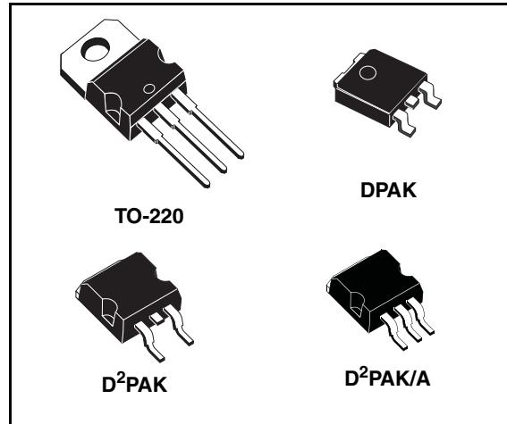
the load, so increase efficiency. Only a 10  $\mu$ F minimum capacitor is need for stability. The device is supplied in TO-220, D<sup>2</sup>PAK, D<sup>2</sup>PAK/A and DPAK. On chip trimming allows the regulator to reach a very tight output voltage tolerance, within  $\pm 1\%$  at 25 °C.
