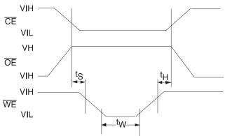
$t_S = t_H = 5 \text{ µsec (min.)}$   $t_W = 10 \text{ msec (min.)}$  $V_H = 12.0V \pm 0.5V$
