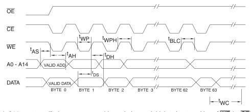
Notes: 1. A6 through A14 must specify the same page address during each high to low transition of  $\overline{\text{WE}}$  (or  $\overline{\text{CE}}$ ).
