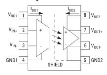
NOTE: A 0.1  $\mu$ F bypass capacitor must be connected between pins 1 and 4 and between pins 5 and 8.
