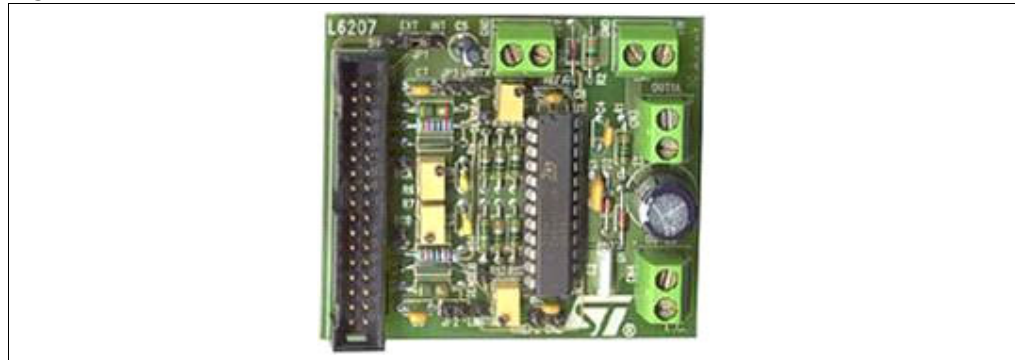
Figure 13. Motor control evaluation board EVAL6207N
