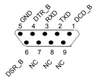
Figure 2-2 SCI Connector J53 Pin Assignments
