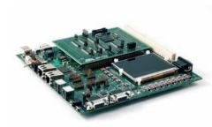
ATSTK1000 provides a complete AT32AP7000 development environment. The kit has two Ethernet ports, a high quality VGA LCD, a loudspeaker, and connectors for USART, PS2, VGA and USB. A expansion header can be used for prototyping.
