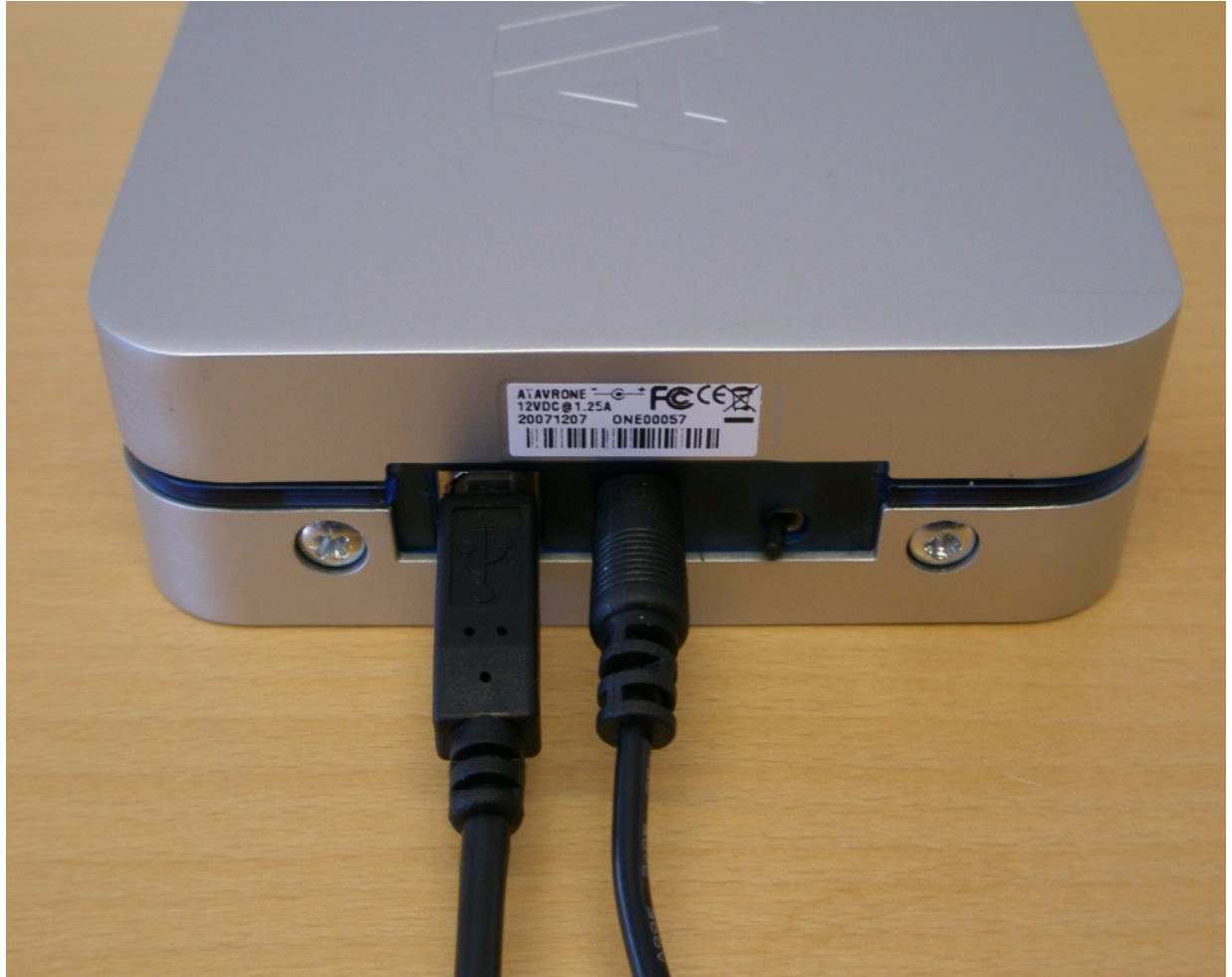
Figure 4-19. AVR ONE! connected to power and USB
