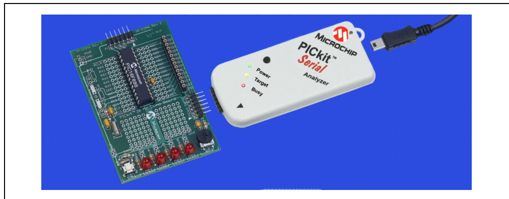
FIGURE 2-1: CONNECTING PICKit™ SERIAL TO THE 28-PIN DEMO BOARD
