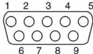
Table 17. CAN D-type 9-pin male connector CN3 and CN4
