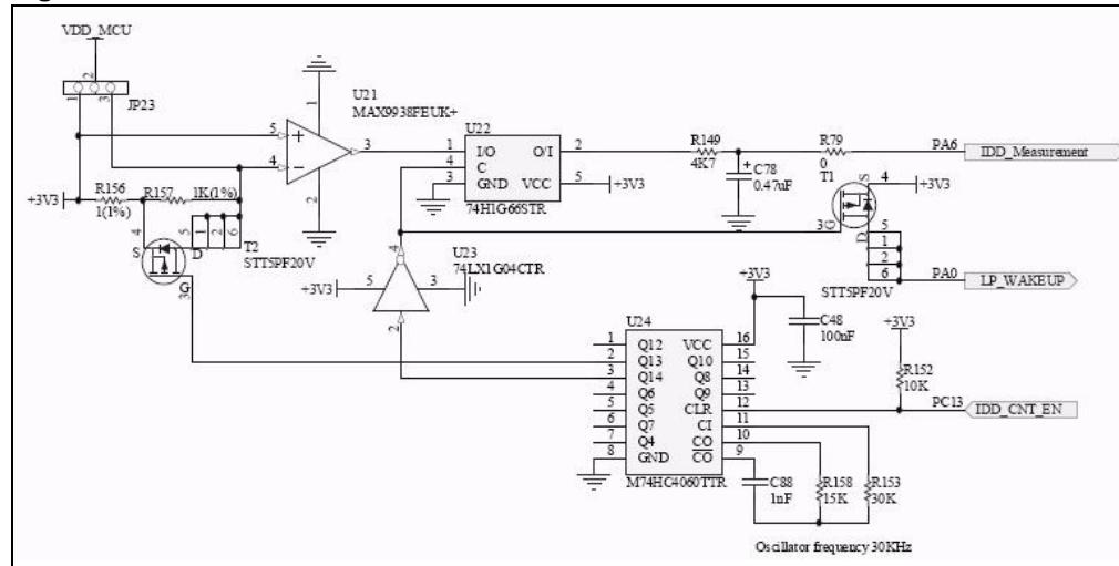
The circuit above is implemented on STM3210C-EVAL for IDD measurement.
