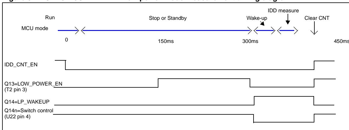
The Low power mode measurement procedure can be used in Stop or Standby modes if the IDD current does not exceed 60  $\mu$ A, otherwise the Run mode measurement procedure should be used up to 60 mA.
