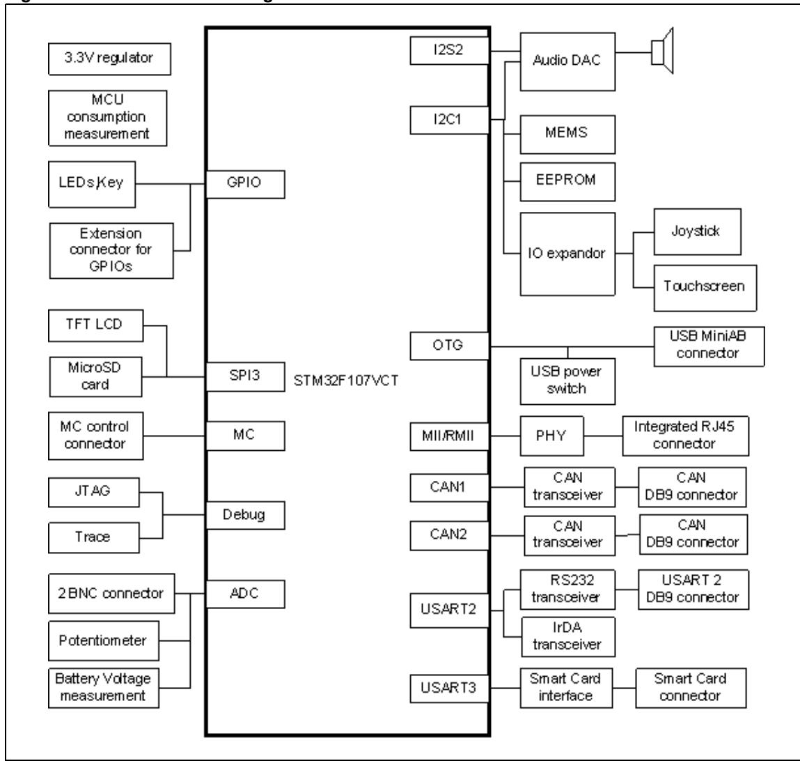
Figure 3. STM3210C-EVAL evaluation board layout
