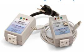
Teridian's Outlet Measurement Unit (OMU) is a compact demonstration kit employing the 78M6612 SOC. The 78M6612 monitors the AC line voltages, frequency, and load current. The embedded firmware calculates items such as RMS line voltage and RMS load current, watts, VA, VAR and power factor. The real time data is transmitted via the serial interface to a PC for display in a Windows® based Graphical User Interface.
