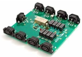
The 78M6618 evaluation board is a design example of a switched 8-outlet power distribution unit with per outlet metering. The board includes one 78M6618 IC, an AC-DC power supply, one AC input, eight switched outputs (relays), and connectors to the serial interfaces and DIO pins.
