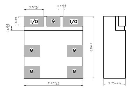
View from below onto the solder terminals and view from beside Marking: 'EPCOS logo' SC 9156, on top of the filter
